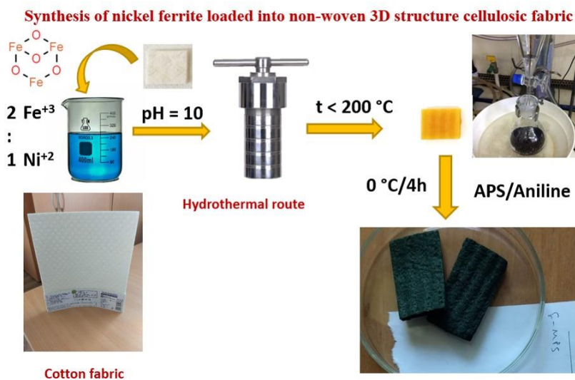
Fig.1 Synthesis of nickel ferrite loaded into non-woven 3D structure cellulosic fabric
